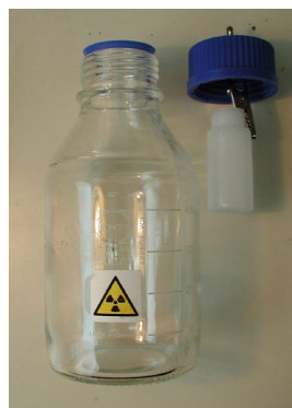
Figure 1. Respirometric flask system: Duran bottle, screw cap, scintillation vial, crocodile clip, threaded rod, wing nut, Teflon liner (Reid et al. 2001)
